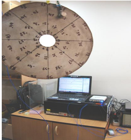
Figure 2. Setup for the experimental modal analysis
